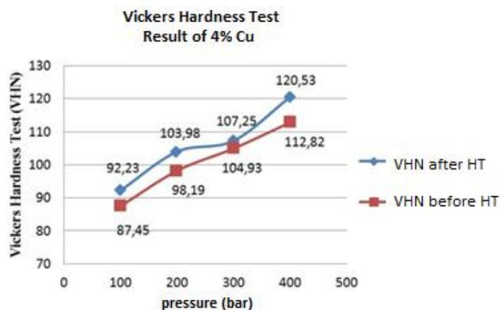
Figure 3. The graph of relationship between pressure squeeze casting with the Vickers test results of 4% cu composition
